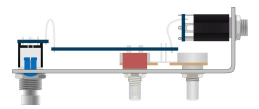
All soldering is completed. Now is a good time to check over the build to make sure no steps were missed and that all connections have been made.
