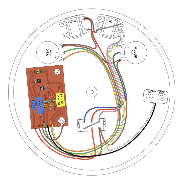
Note: The battery wiring has been updated to use a TRS jack but otherwise all wiring matches vintage units. Check the pinout of your chosen transistors before soldering. P-PC-FUZZ-ISS2-BRN boards are available at www.amplifiedparts.com.
